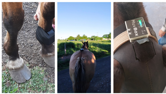
Fig. 2: Image of the proposed system. Inertial devices on the head, limb, and pelvis.
